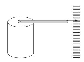
Cut the neck off of the balloon and stretch it over the open end of the coffee can. Use the rubber band to hold it in place. Make sure there are no leaks, using glue if necessary.
