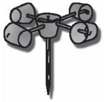
Punch one hole per cup in 4 of the cups. Punch 4 holes, equally spaced, around the edge of the 5th cup. Also cut the bottom out of this cup. Slide the straws through the four punched holes so they form a cross. Put a cup on each straw end, and aim them all either clockwise our counterclockwise. Glue in place. Push the pin through the crossing point of the straws and down into the pencil eraser. You have now created a axis cup anemometer! **How to measure wind speed:**
