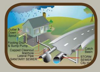
If you are connected to the sanitary sewer, all household wastewater flows to a wastewater treatment plant, where it is cleaned. Storm water is kept separate from our sanitary wastewater.
